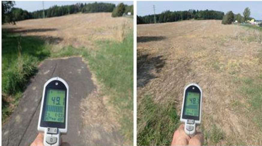
Figure 5: Surface temperature (ST) measurements on 26 August 2017, incoming solar energy approx. 700\text{W}/\text{m}^2 . The ST of a harvested field ( 48^\circ\text{C} ) nearly equals that of an asphalt surface ( 49^\circ\text{C} ).
